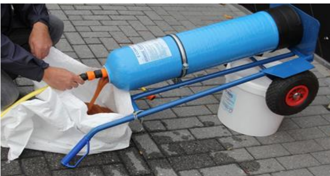
5. look if all the resin is out of the bottle, if not, rinse bottle with clean water using a garden hose with nozzle
