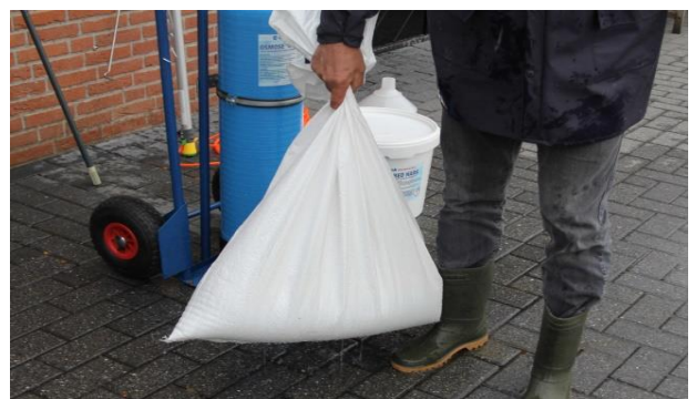
6. drained resin (plastic granules) in a water-permeable bag can be completely disposed of with plastic waste
