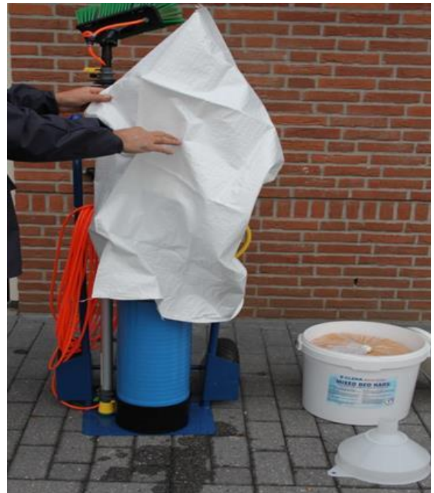
2. place the supplied water-permeable bag over the opening of the bottle
